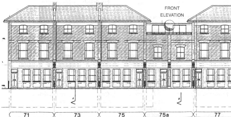
Plans of the original front elevation for 71-77 Upper Brockley Road by Architecture Limited. There may be some modifications by the newly appointed architects.
